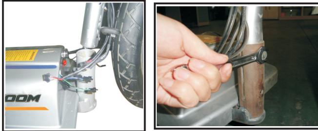
4. Tighten the bolts and nuts by the allen wrench provided in the tool kit.
