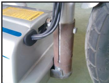
6. Ensure that the handlebar is facing front before tightening using the allen wrench provided.
