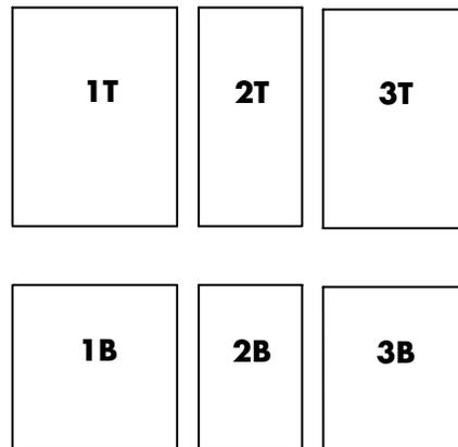
Note: 1B/1T panels always go on the left side of the back wall. 2B/2T panels always go on the right side of the back wall.
