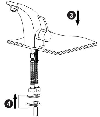
Insert waterlines 3 and fixing bolt 2 into the set hole of the under mount sink or 1 3/8" drilled hole of the counter top. Put on the rubber washer 5 and brass washer 6 then securely tighten with nut 7. Place the faucet body 1 and use the spanner to tighten the nut 7 securely.
