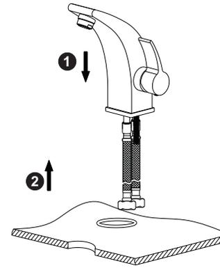
Screw waterlines 3 into the inlet pipe of the faucet body 1. Fit o-ring 4 into the bottom groove of Faucet body 1.
