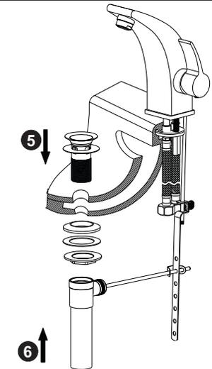
Insert the drain-off pole 10 through the hole of the basin. Tighten the drain-off pole 10 securely. Place the end side of the lift pole 9 through the drain-off pole 10 and then tighten the screw.
