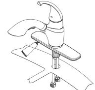
Place putty beneath the plastic gasket and install faucet through center hole.
