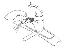
Remove spray head hose line. Turn on water and check for leakage. Řeplace spray head.
