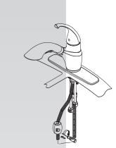
Attach metal weight to the hose to prevent hose from twisting. Return hose to proper position.
