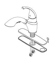
Attach cover plate to bottom of faucet with plastic gasket.
