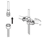
Tighten end of shank with wrench and slip hose into the inlet port.
