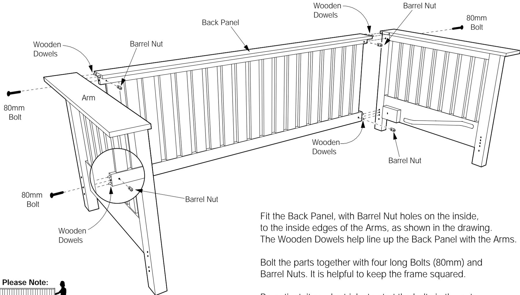
Fit the Back Panel, with Barrel Nut holes on the inside, to the inside edges of the Arms, as shown in the drawing. The Wooden Dowels help line up the Back Panel with the Arms.
