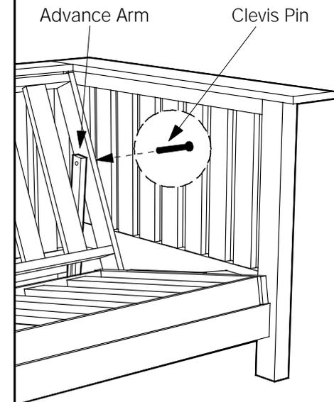
Secure with a Washer and Locking Pin.
