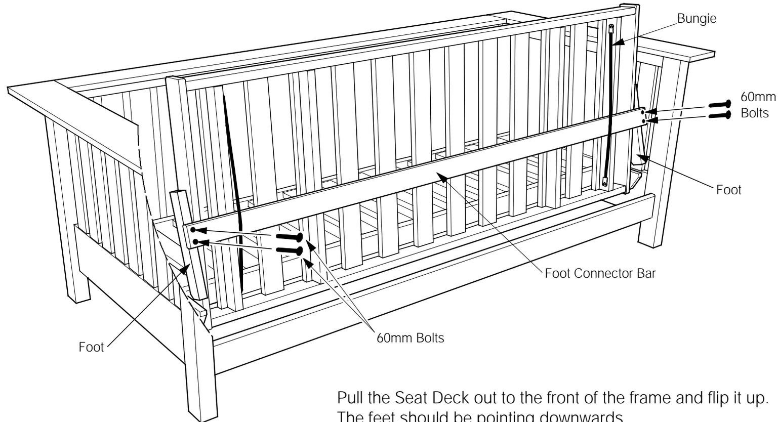
Pull the Seat Deck out to the front of the frame and flip it up.
