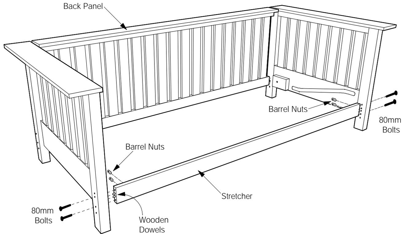
Fit the Stretcher, with the Barrel Nut holes on the inside, to the inside edge of the Arms.
