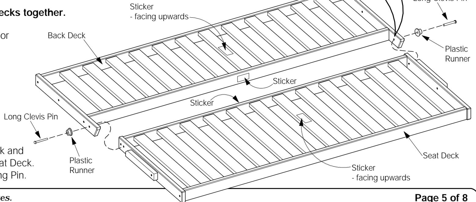
The Seat Deck fits inside the Back Deck as shown. Slip the Long Clevis Pin through the small end of the Plastic Runner, through the hole in the Back Deck and the corresponding hole in the Seat Deck. Secure with a Washer and Locking Pin.
