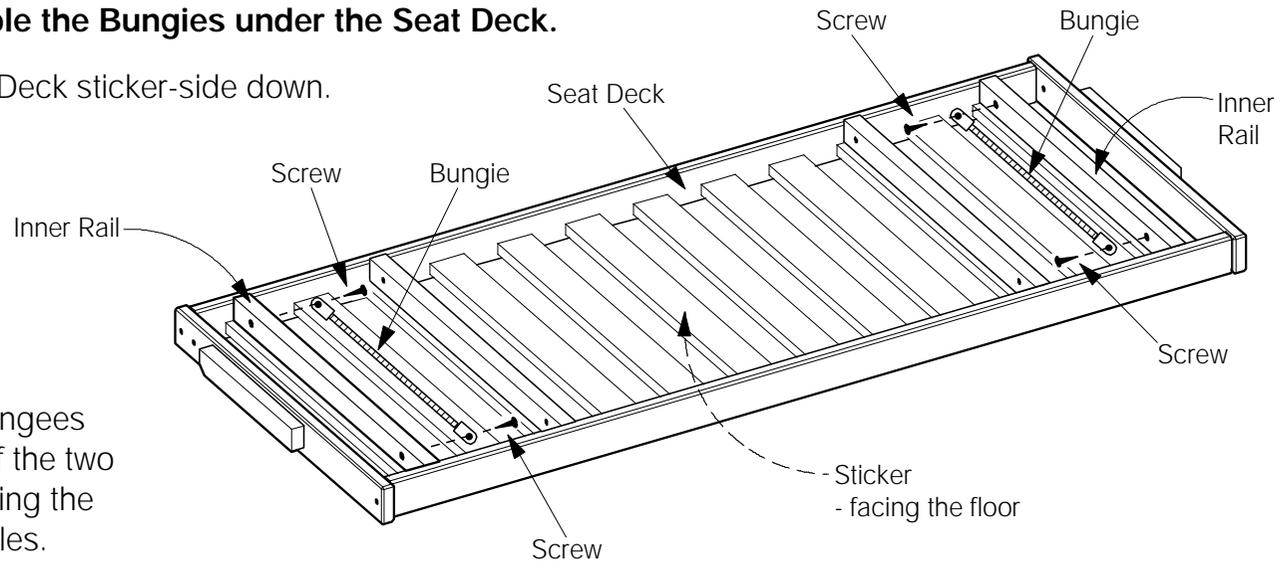
Screw the Bungies to the side of the two inner rails, using the pre-drilled holes.
