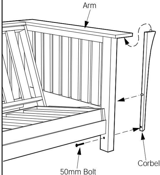
Secure with a short Bolt (50mm) from the inside of the Arm at the bottom. Tighten until the Corbel is snug.
