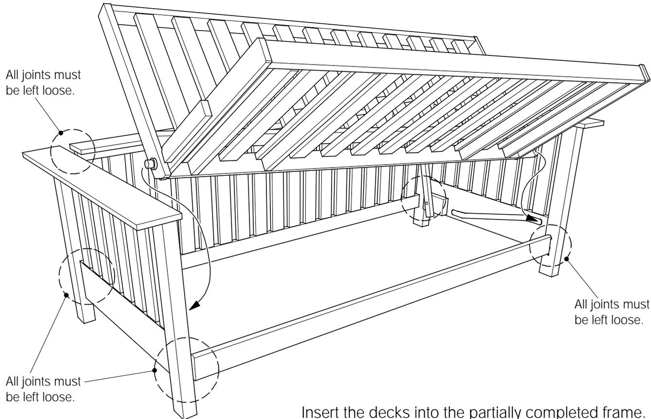
Insert the decks into the partially completed frame. This is where a helper may be useful.
