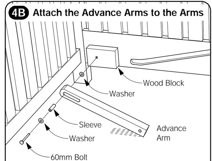
The slotted end of the Advance Arm attaches to the little wood block at the back of the Arm. Slip a washer and Sleeve over the Bolt, and pass it through the slot. Add another washer and fix it to the Arm. Tighten the Bolt. Be sure that the Advance Arm moves freely. Rotate the Advance Arm so that is pointing up.
