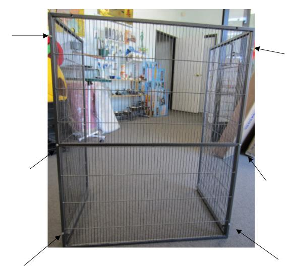
Then, proceed to attach the cage front to the two remaining sides.
