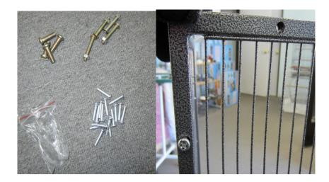
When you are done attaching the sides to the cage rear it should look similar to this. Make sure that there is a screw securely in place for each vertical hole.
