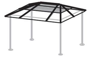
Remove protective plastic from both sides of upper roof panels (13,14,15). Place side to face toward the sun facing out when installing.
