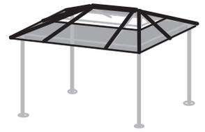
Remove protective plastic from both sides of lower roof panels (17,18,19). Place side to face toward the sun facing out when installing.
