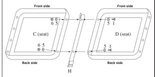
Place the flat metal bar (H) with hook in one end and connect two seat panels with bolt (1) and washer (5) and nut (6) on other side.
