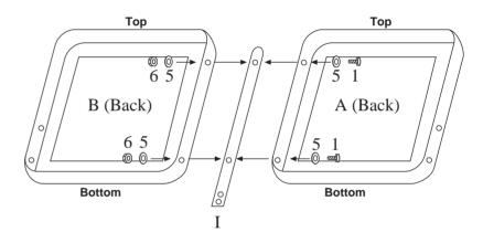
Place the flat metal bar (I) in one end and connect two back panels with bolt (1) and washer (5) and nut (6) on other side.
