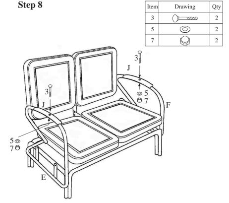
Carefully line up the holes in arm cover (J) with holes on arm frame (E/F), using a quick downward push, snap cover over frame. Attach arm holder to each side frame with the bolt (4). Then washer (5) and round top nut (7) should be used underneath the arm cover. Assemble as shown.
