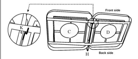
Turn the connected seat panel over and place the seat frame support (K) on the bottom of the seat as shown in diagram. Secure the seat frame support with the seat panel with bolt (1), washer (5) and nut (6).
