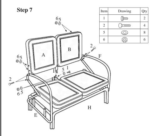
Plug the seat back's center bar (I) into the hole of center bar (H) on seat bottom. Tighten the bar with bolt (1) washer (5) and nut (6).
