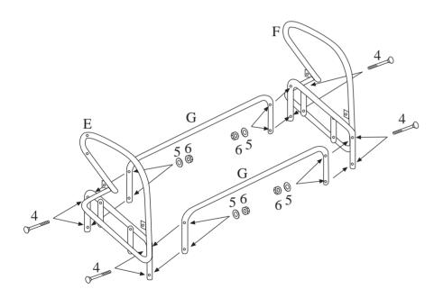
Attach the two side frames on connecting tube (G) on both sides with bolt (4) on the outside, washer (5) and nut (6) on the inside. Assembles as shown.
