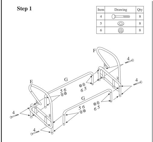
Attach the two side frames on connecting tube (G) on both sides with bolt (4) on the outside, washer (5) and nut (6) on the inside. Assembles as shown.
