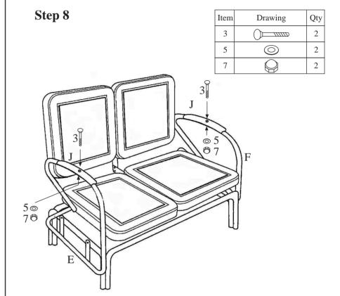
Carefully line up the holes in arm cover (J) with holes on arm frame (E/F), using a quick downward push, snap cover over frame. Attach arm holder to each side frame with the bolt (4). Then washer (5) and round top nut (7) should be used underneath the arm cover. Assemble as shown.
