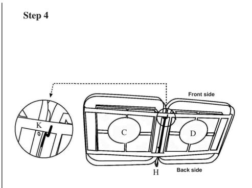
Turn the connected seat panel over and place the seat frame support (K) on the bottom of the seat as shown in diagram. Secure the seat frame support with the seat panel with bolt (1), washer (5) and nut (6).
