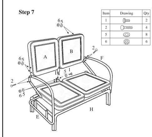
Plug the seat back's center bar (I) into the hole of center bar (H) on seat bottom. Tighten the bar with bolt (1) washer (5) and nut (6).
