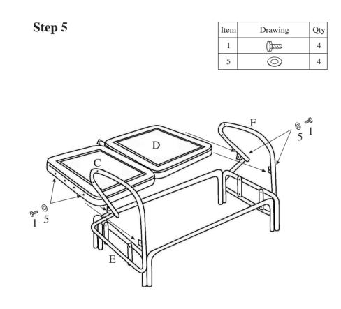
Attach the seat bottom on arms with bolt (1) and washer (5). Assembles as shown.
