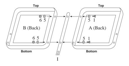
Place the flat metal bar (I) in one end and connect two back panels with bolt (1) and washer (5) and nut (6) on other side.
