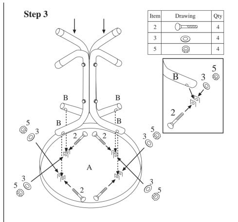
Put the table top (A) on the leg assembly (B) and then fix it with screw (2), washer (3) & nut (5). Assemble as shown.
