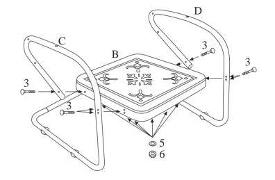
Attach the seat bottom (B) to side frame on both sides with screw (3) on th outside, washer (5) and nut (6) on the inside. Assemble as shown.
