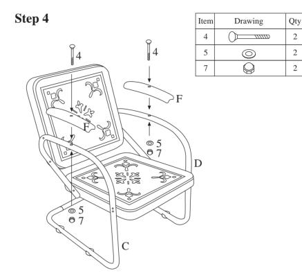
Carefully line up holes in arm cover (F) with holes on chair frames. Using a quick downward push, snap cover over frame. Attach arm holder (F) to each side frame with the bolt (4).
