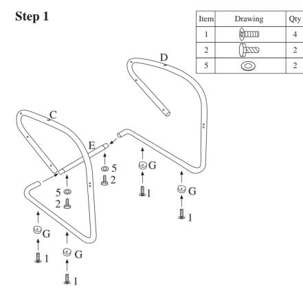
Attach the four rubber feet (G) at the bottom of the arm side frames (C/D) with screws (1) as shown. Insert the rear connecting tube (E) to each of the arm side frames (C/D) as shown.
