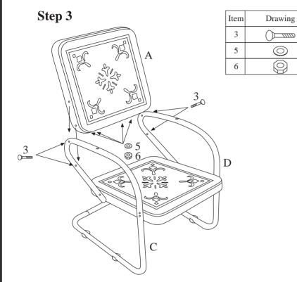
Attach the seat back (A) to side frames, on both sides with bolt (3) on the outside, washer (5) and nut (6) on the inside. Assemble as shown.
