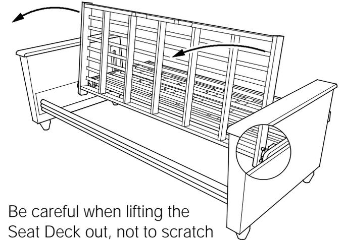
Be careful when lifting the Seat Deck out, not to scratch the Arms with the Rollers.
