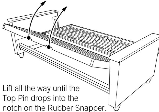
Lift all the way until the Top Pin drops into the notch on the Rubber Snapper.
