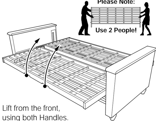
Lift from the front, using both Handles.
