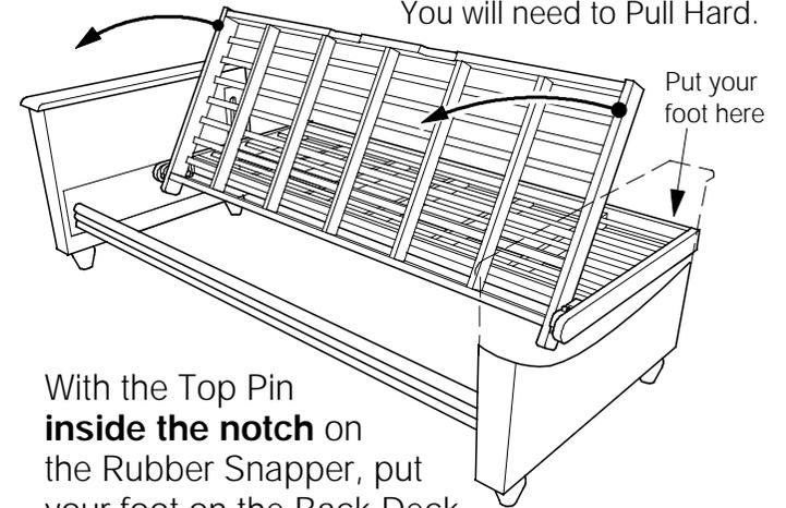
With the Top Pin **inside the notch** on the Rubber Snapper, put your foot on the Back Deck and pull the Seat over the "Snap Point"
