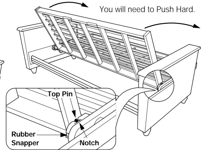
**5D** From the Back, lift out the Top Pin and ease the Seat Deck forward.
