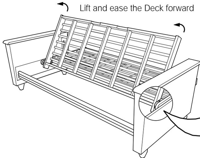
Lift up so the Top Pin is out of its notch in the Rubber Snapper. Ease the Back Deck forward, keeping it orientated vertically.
