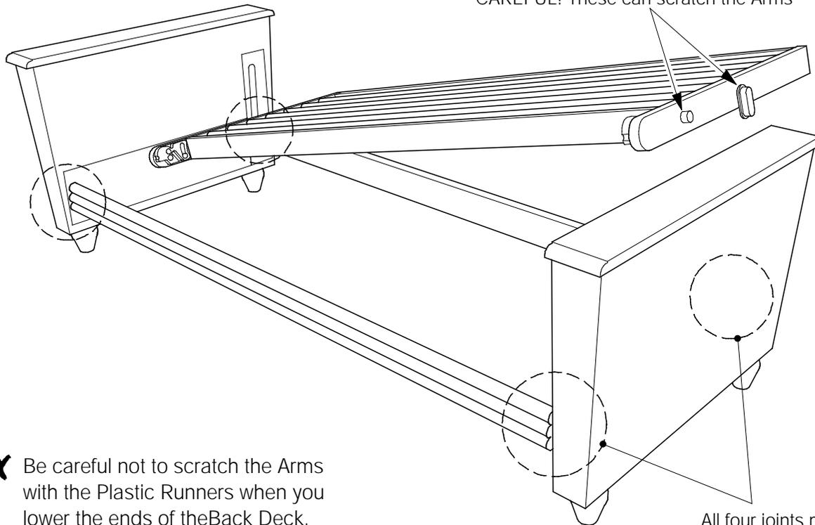
**X** Be careful not to scratch the Arms with the Plastic Runners when you lower the ends of the Back Deck.
