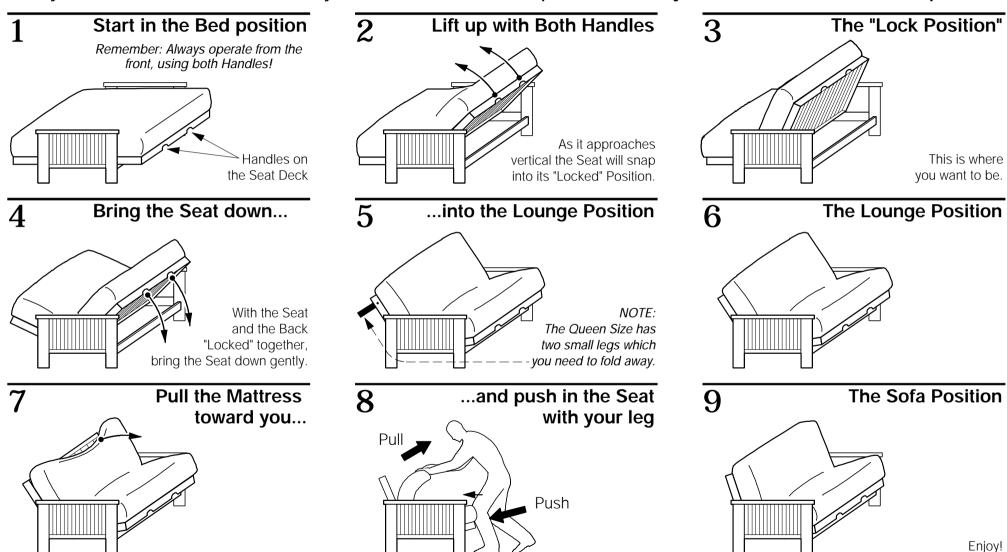
Filease Note: If the rollers of the mechanism become improperly disengaged, the Back Deck could come down more quickly than you expect!
