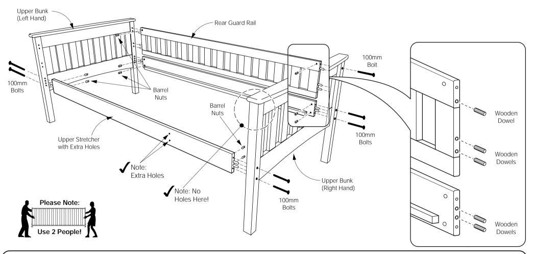
5A Attach the Front Guard Rail to the Upper Bunk.
