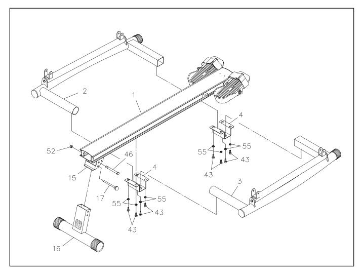
**NOTE:** Lay your partially assembled **1215 Orbital Rower** up side down to complete STEP 3 and 4.
