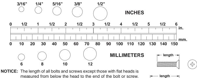
measured from below the head to the end of the bolt or screw. Flat head bolts and screws are measured from the top of the head to the end of the bolt or screw.
