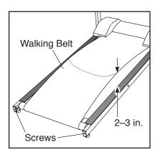
rear roller adjustment screws counterclockwise 1/4 of a turn. When the walking belt is properly tightened, you should be able to lift each edge of the walking belt 2 to 3 in. (5 to 7 cm) off the walking platform. Be careful to keep the walking belt centered. Walk on the treadmill for a few minutes. Repeat until the walking belt is properly tightened.
