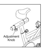
Make sure that the adjustment knob is engaged in an adjustment hole.
