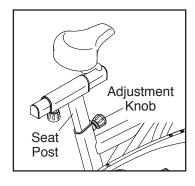
the adjustment knob. Make sure that the adjustment knob is engaged in an adjustment hole.
