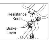
To stop the flywheel, push the brake lever downward. The flywheel should quickly come to a complete stop.
