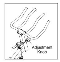
ment knob. Make sure that the adjustment knob is engaged in an adjustment hole.
