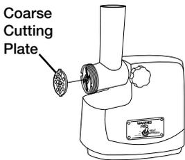
4. Place the coarse cutting plate in the grinder/feeder head.
