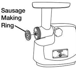
10. Insert sausage-making ring into feed screw. Make sure notch on sausage making ring aligns with notch in feed screw.
