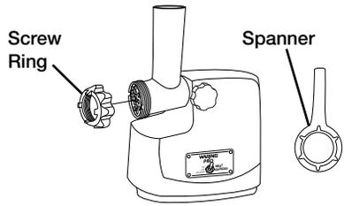
5. Tighten screw ring onto the grinder/feeder head. Use spanner to secure screw ring.
