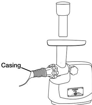
12. Slide casing over the end of the sausage attachment, leaving approximately 2" overhanging the end of the attachment.
