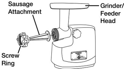
11. Put the desired sausage attachment (small or large) into screw ring and screw onto the grinder/feeder head. Use spanner to secure screw ring.
