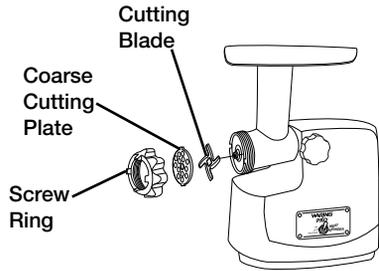
9. Once meat has gone through grinder, turn unit off. Remove screw ring, coarse cutting plate and cutting blade.
