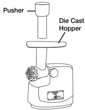
6. Place large die-cast hopper onto grinder/feeder head.
