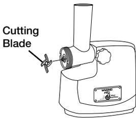
3. Assemble cutting blade on the end of the feed screw with flat cutting surface facing away from the feed screw.
