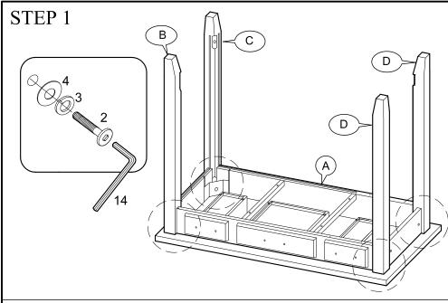
Place the top frame upside down on soft surface. Align and fasten left, right front and right rear legs to top frame using short bolt, lock washer and flat washer and tighten with Allen wrench.
