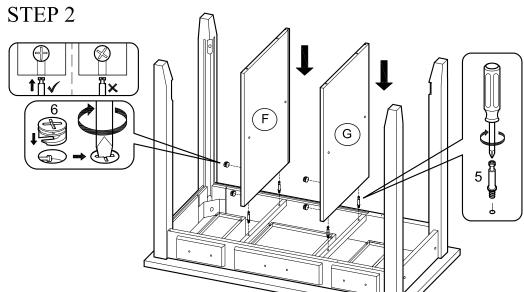
Screw in cam bolt to top frame using screw driver (Not Included) as shown in the diagram. Align the cam bolt with pre-drilled holes on left and right divider then insert cam nut into pre-drilled holes on the left and right divider and tighten with screw driver (Not Included) as shown in the diagram.
