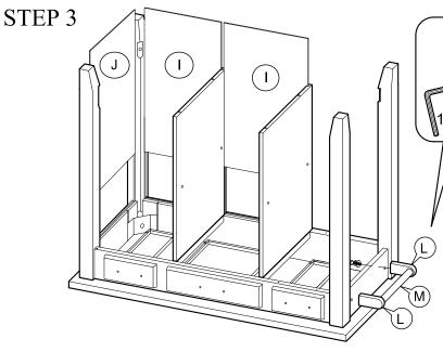
Insert rod to brackets then align and fasten brackets to top frame using medium bolt, lock washer and flat washer and tighten with Allen wrench.
