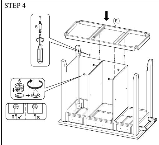
Screw in cam bolt to bottom frame using screw driver (Not Included).
