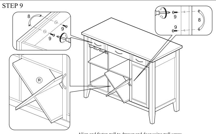
Align and fasten pull to drawer and door using pull screw. Assemble the wine rack panels together then place into the server as shown.
