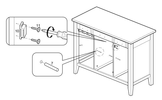
Align and fasten magnetic catch to right divider using flat head screw. Insert shelf support to left and right divider and left legs.
