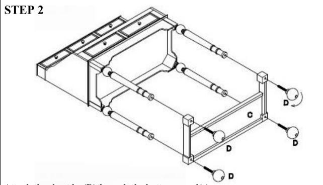
Attach the short leg(D)through the bottom panel(c)
