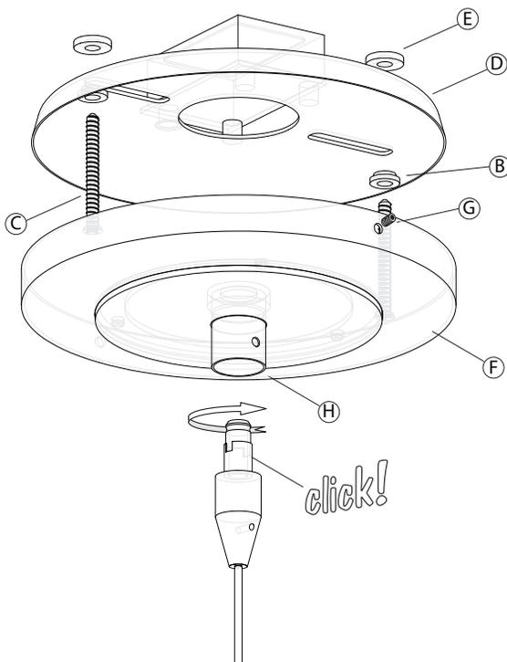
The 4" Surface Mount Canopy can be mounted directly to any wall or ceiling with access to the power cables. Begin by connecting the two wires from the transformer (A) to the power cables in the wall. Then slide the notched plastic washer (B) through the mounting screw (C). Insert the screw (C) into the mounting plate (D) and slide the plastic washer (E) onto the end of the screw. Align the screws (C) with the J-box and tighten until firmly connected.
