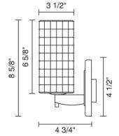
Suitable for dry locations only Mount to 3 1/2" - 4" round J-box Short circuit protection Overload protection Thermal protection
