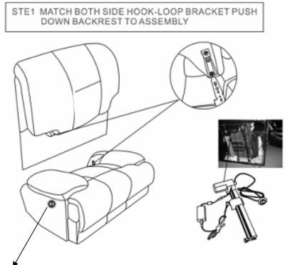
Press the button to control the power mechanism.
