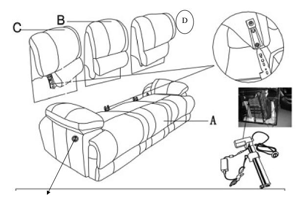
Press the button to control the power mechanism.
