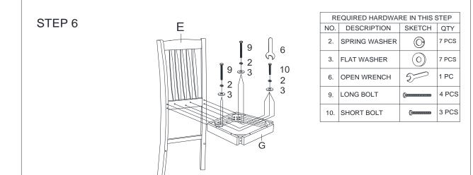
Attach seat frame (G) to chair back frame (E) using short bolts (10), long bolts (9), spring washers (2) and flat washers (3) as shown. do not tighten the bolts in this step.
