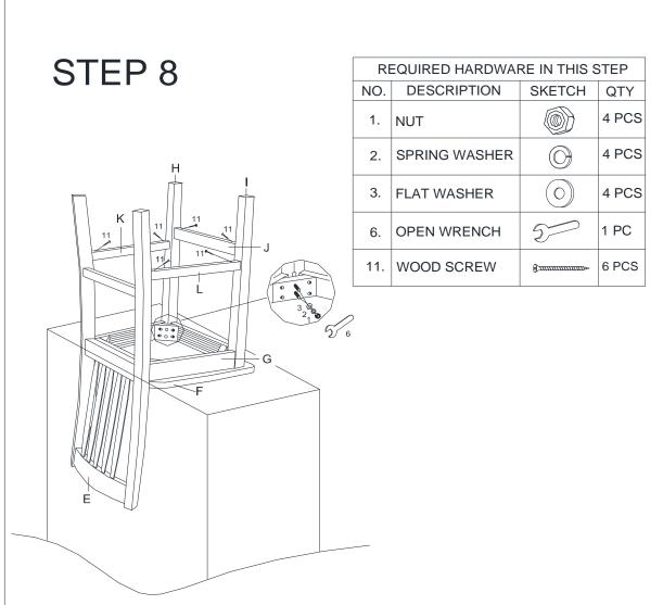
Attach chair left and right front legs (H & I) to seat frame (G) with flat washers (3), spring washers (2), and nuts (1) as shown. Do not fully tighten nuts (1). Insert chair left side crossbar and chair right side crossbar (K & L) into the front left and right chair legs (H & I) and chair back frame (E).
