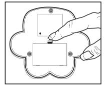
2. Insert one 9-V battery. Reattach compartment cover.
