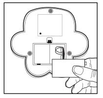
3. If your Pet Paw will not activate your Pet Chime, use a small screwdriver to fine tune the sensitivity by turning within 1mm clockwise or counter-clockwise while pressing the Paw repeatedly until you hear that the Pet Chime is activated. (see diagram below).
