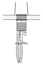
3. Screw the spray hose to the spray hose pipe.
