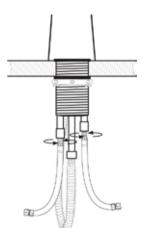
4. Attach the male ends of the flexable hoses to the hot and cold brass pipes on the faucet body. Then connect the female ends of the flexable hose to the corrosponding hot & cold water supply.
