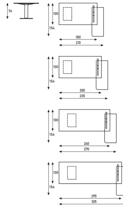
Bridge Desk is a combination of desk and a matching supporting cupboard. Creating a spacious surface with a closed storage element. The cupboard, which is partly placed under the desk, has an aluminium roller door. Together with the desk, this gives the Bridge a sober, restful appearance. Perfect for every office, Bridge Desk is available in four sizes.
