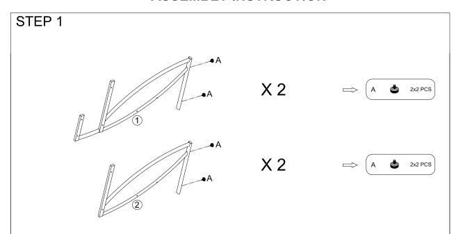
Insert (A) Floor Levelers into the BOTTOMS of (1) Main Desk Frames and (2) Computer Desk Frames as shown.
