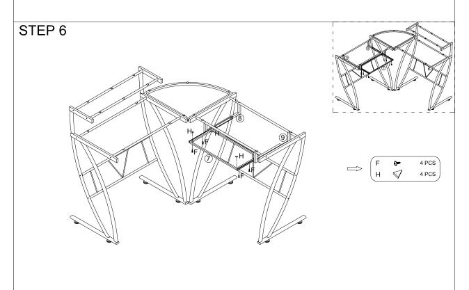
1. Extend the Keyboard Glides and set (7) Keyboard Frame in place as shown. Secure from UNDERNEATH with (F) 4
