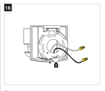
2 Remove the mounting plate by pulling the bottom of the mounting plate out and then down.
