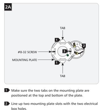
**3** Level the mounting plate vertically and secure it to the electrical box with the two #8-32 screws provided.
