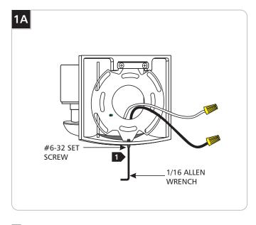
Loosen (**Do Not Remove**) the #6-32 set screw at the base of the sconce with the provided 1/16 Allen wrench.
