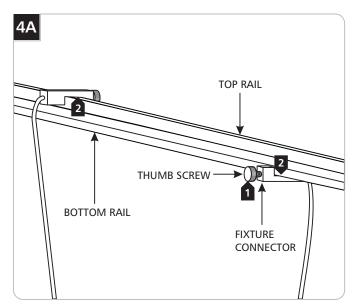
**NOTE:** One fixture connector must be mounted on the top rail and the other one on bottom rail.
