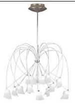
Fifteen whimsical arms wrapped from a central core, each tipped with a frosted lamp and white flight paper. 9" diameter round canopy houses a 300 watt electronic transformer with short circuit protection. Includes fifteen 12 volt, 20 watt Frostlineâ,,¢MR16 lamps. Dimmable with a lowvoltage electronic dimmer.
