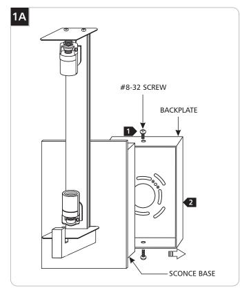
Remove the two #8-32 screws on the backplate with a Phillips head screwdriver. BACKPLATE FLECTRICAL BOX TOTAL STREET TOT
