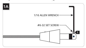
1 Back out (do not remove) the #6-32 set screw on tip of the connector with the provided 1/16 Allen wrench.
