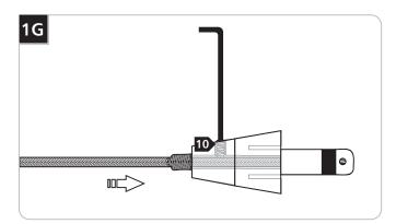
Tighten the #6-32 oval head set screw on the conical connector firmly.
