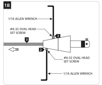
Backout (do not remove) the two #6-32 oval head set screws on the conical connector with the provided 1/16 Allen wrench.
