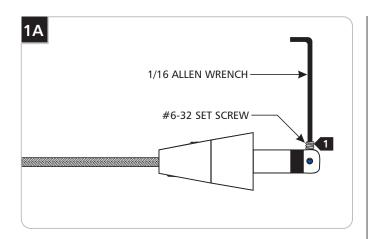
Back out (do not remove) the #6-32 set screw on tip of the connector with the provided 1/16 Allen wrench.
