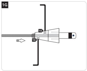
Tighten the two #6-32 oval head set screws on the conical connector firmly.
