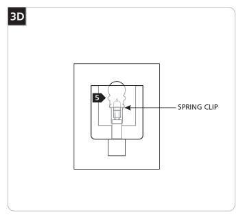
5 Push the lamp shield onto the spring clip.
