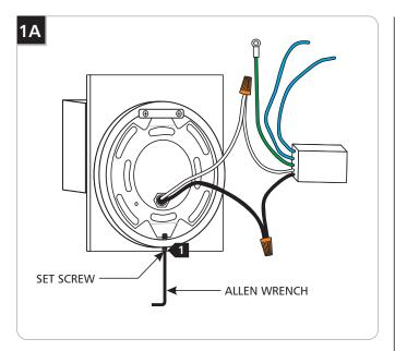
1 With the Allen wrench provided, back out (do not fully remove) the set screw at the base of the sconce.
