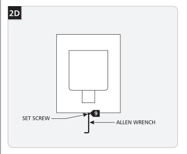
2 Line up the sconce on the wall and then secure the sconce to the mounting plate by tightening the set screw at the base of the sconce.
