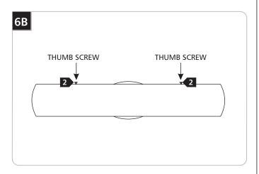
2 Tighten the two thumb screws on one side of the back plate.
