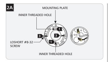
Make sure the two inner threaded holes on the mounting plate are positioned vertically.
