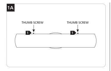
**1** Loosen (do not remove) the two thumb screws on one side of the fixture.
