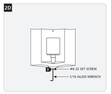
2 Level the sconce vertically and secure it to the mounting plate by tightening the #6-32 set screw at the base of the sconce with the 1/16 Allen wrench.
