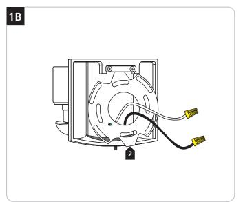
Remove the mounting plate by pulling the bottom of the mounting plate out and then down.
