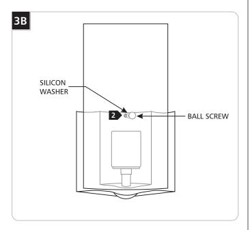
2 Tighten the provided ball screw and silicon washer through the glass shade hole into the sconce base screw hole to secure the glass shade in place.
