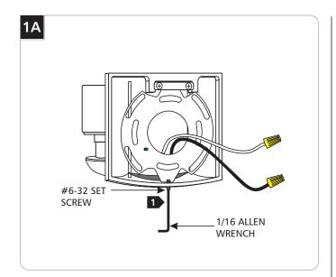
1 Loosen (Do Not Remove) the #6-32 set screw at the base of the sconce with the provided 1/16 Allen wrench.
