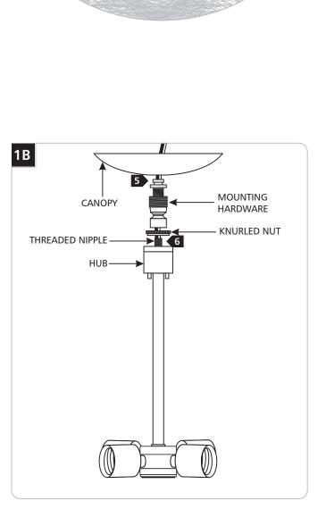
Feed fixture wires through the knurled nut, mounting hardware and canopy respectively.
