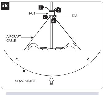
**NOTE:** Make sure to support the glass shade while adjusting the aircraft cables to position it in place as described in the steps below.
