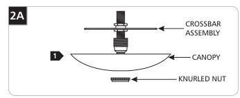
Loosen the knurled nut to remove the canopy from the crossbar assembly.
