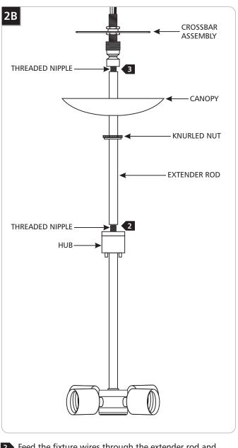
2 Feed the fixture wires through the extender rod and tighten it completely to the threaded nipple attached to the fixture hub.
