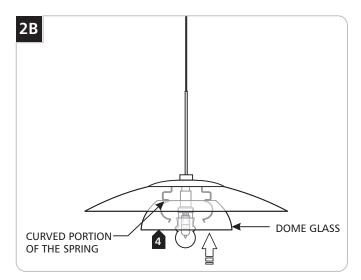
4 Push the dome glass onto the three springs so that it rests behind the curved portion of the springs.
