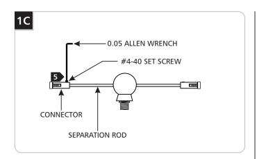
Replace the connectors at the end of the separation rods and tighten the #4-40 set screw with the 0.05 Allen wrench.
