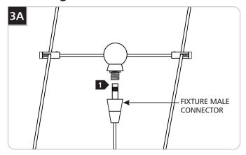
Screw the fixture FreeJack male connector into the Kable Lite FreeJack connector tight.
