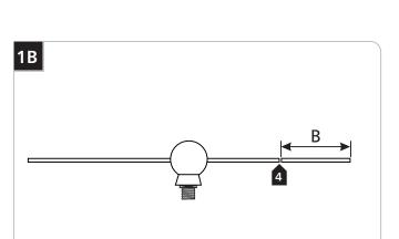
4 Use a sharp cutter or a hacksaw to cut the separation rods.
