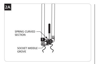
1 Snap the spring curved section into the socket middle groove.
