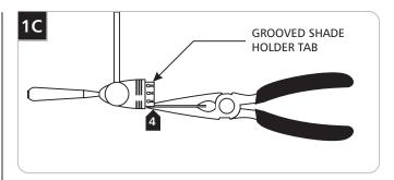
4 If the Lil Egypt fits tight onto the fixture, then carefully bend the grooved shade holder tabs in slightly with the needlenose pliers. If it fits loose, then carefully bend the grooved shade holder tabs out slightly with the needlenose pliers.
