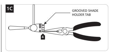
If the Tinkerbell fits tight onto the fixture, then carefully bend the grooved shade holder tabs in slightly with the needlenose pliers. If it fits loose, then carefully bend the grooved shade holder tabs out slightly with the needlenose pliers.
