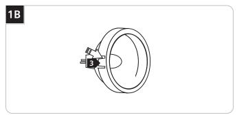
Use MAX 50 Watt MR16 Front Cover Halogen Lamp, except for Antique Bronze & Black Finishes Use MAX 35 Watt MR16 Front Cover Halogen Lamp.
