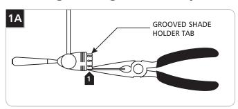
If the Sugar accessory fits tight onto the fixture, then carefully bend the grooved shade holder tabs in slightly with the needlenose pliers. If it fits loose, then carefully bend the grooved shade holder tabs out slightly with the needlenose pliers.
