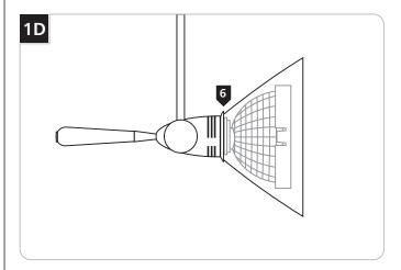
6 Hold the lamp against the glass with the thumb and push the lamp pins all the way into the socket holes; simultaneously push the Sugar accessory metal ring onto the grooved shade holder.
