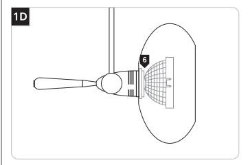
6 Hold the lamp against the shade with the thumb and push the lamp pins all the way into the socket holes; simultaneously push the Meteorite shade metal ring onto the grooved shade holder.
