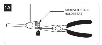
If the Meteorite shade fits tight onto the fixture, then carefully bend the grooved shade holder tabs in slightly with the needlenose pliers. If it fits loose, then carefully bend the grooved shade holder tabs out slightly with the needlenose pliers.
