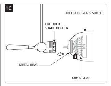
Place the MR16 lamp into the Dichroic Glass Shield.
