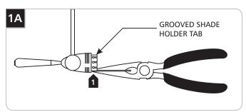
If the Dichroic glass Shield fits tight onto the fixture, then carefully bend the grooved shade holder tabs in slightly with the needlenose pliers. If it fits loose, then carefully bend the grooved shade holder tabs out slightly with the needlenose pliers.
