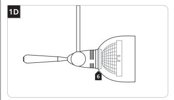
6 Hold the lamp against the Dichroic Glass Shield with the thumb and push the lamp pins all the way into the socket holes; simultaneously push the Dichroic Glass Shield metal ring onto the grooved shade holder.
