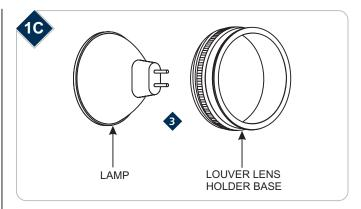
Place the lamp into the louver lens holder base.
