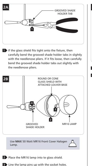
Push the lamp pins all the way into the socket holes; simultaneously push the glass shield onto the groove shade holder.
